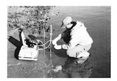
Figure 2-2 Direct-Push Sample Collection Using a T-Handled Probe
