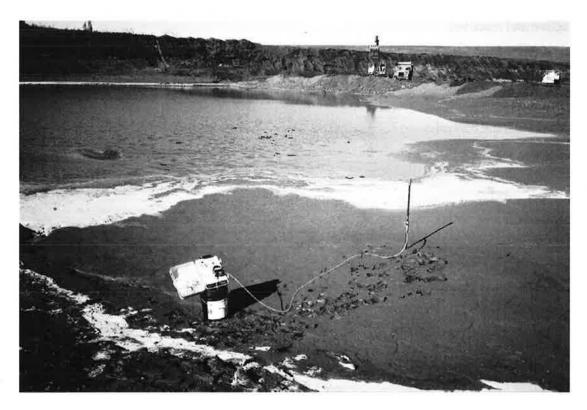
Figure 2-1 Direct Push Sample Collection Using a Drive Point Piezometer
